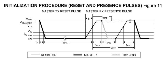
After the bus master has released the line it goes into receive mode (RX). Now, the 1-Wire bus is pulled to  $V_{PUP}$  via the pullup resistor or, in case of a DS2480B driver, by active circuitry. When the threshold  $V_{TH}$  is crossed, the DS1963S waits for  $t_{PDH}$  and then transmits a Presence Pulse by pulling the line low for  $t_{PDL}$ . To detect a presence pulse, the master must test the logical state of the 1-Wire line at  $t_{MSP}$ .
